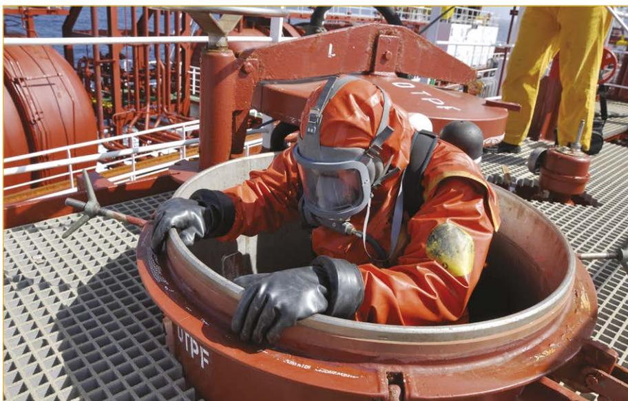
'Tank cleaning can be performed by the ship's crew and/or by employing a riding crew. If the cleaning is done by the crew it would likely take a minimum of four days per tank and if using a riding crew to clean the tanks this could come down to two days'
